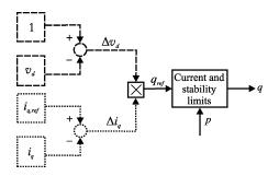
Fig. 16. Block diagram used for reactive power regulation: the reference signal  $q_{\rm ref}$  is obtained from error terms  $\Delta v_d$  and  $\Delta i_q$ .
