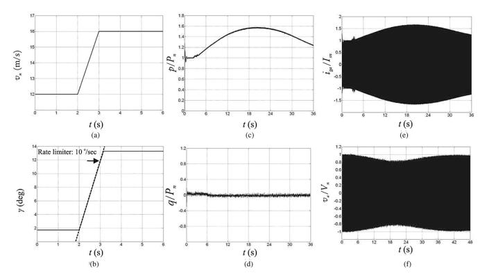
Fig. 15. Case study B, oscillograms: (a) wind speed, (b) pitch angle, (c) normalized active power, (d) normalized reactive power, (e) normalized grid current, and (f) normalized voltage measured at the PCC.
