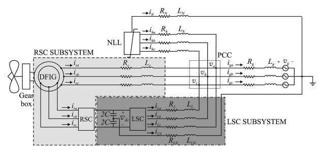
Fig. 2. System configuration: the DFIG stator is connected to the PCC; DFIG rotor is supplied by two back-to-back connected converters; the dc-link central tap is tied to the neutral. NLL is connected to the PCC. The step-up transformer and the supply line are represented by means of their Thevenin equivalent.
