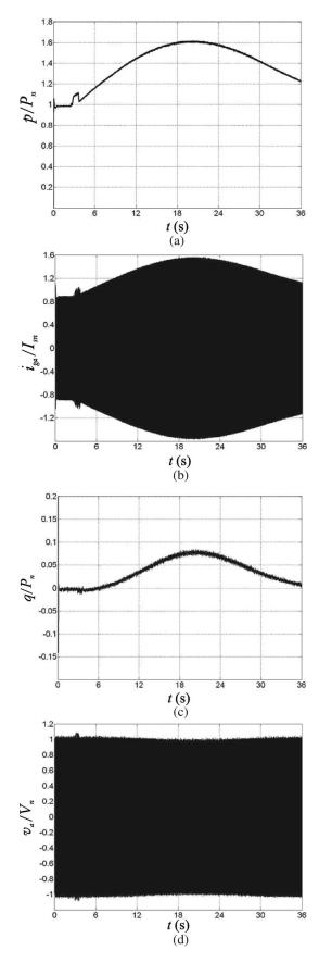
Fig. 17. Case study B, reactive power compensation is implemented: (a) normalized active power, (b) normalized reactive power, (c) normalized grid current, and (d) normalized voltage at the PCC.
