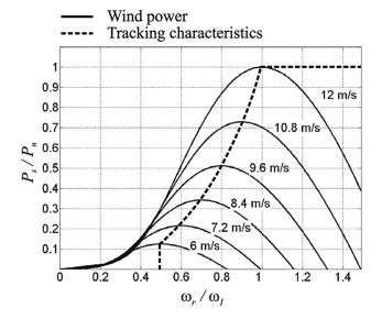
Fig. 1. Wind turbine tracking characteristic: the target normalized stator power for different wind speeds versus normalized rotor speed.
