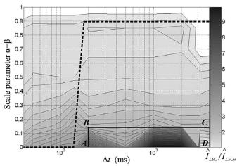
Fig. 11. Symmetrical sag: normalized LSC peak current contour plot. x-axis:  $\Delta t$  (ms); y-axis: scale parameter  $\alpha=\beta$ .
