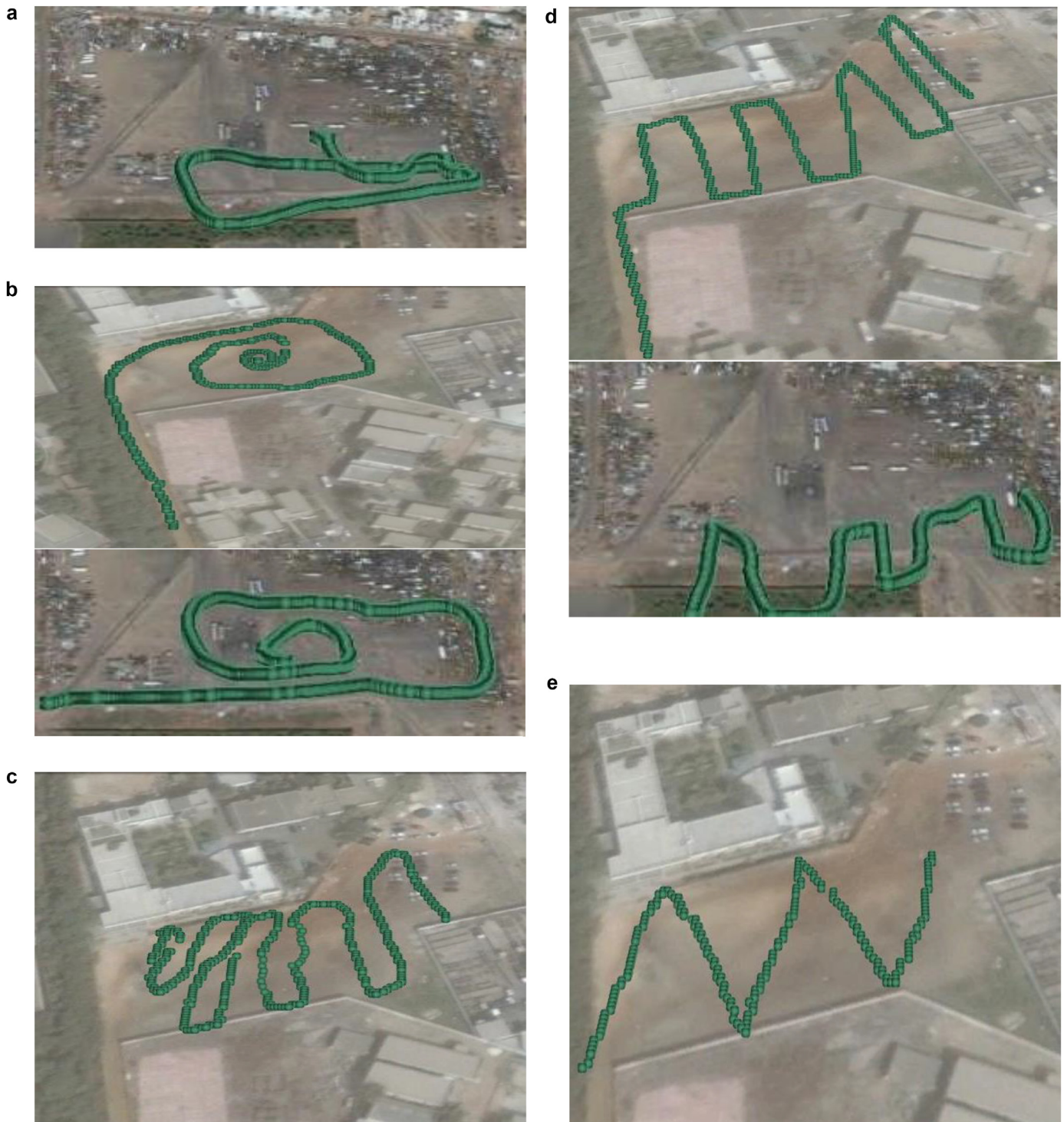
Fig. 13. (a) Picture of covered random paths, (b) Pictures of covered spiral paths, (c) Pictures of covered zigzag paths, (d) Pictures of covered rectangular function paths, (e) Pictures of covered sawtooth wave model paths.
