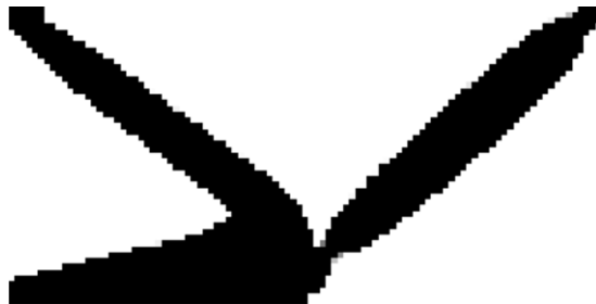
Fig. 6b. The optimized design of the compliant mechanism without length scale control.
