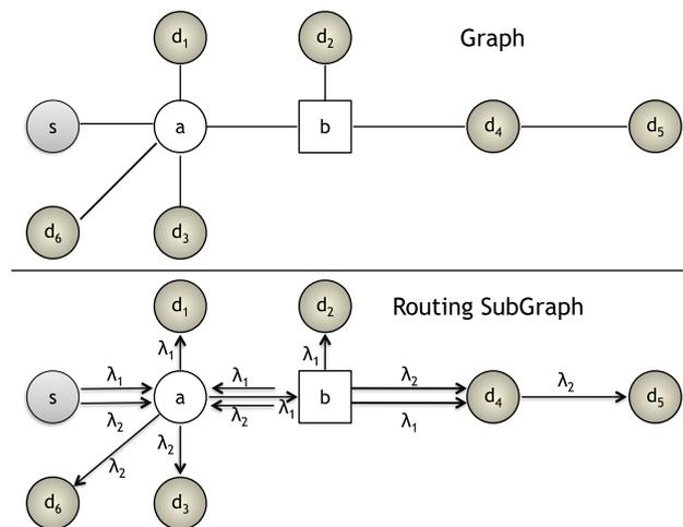
Fig. 4. Network example illustrating the problem assumptions (MC nodes are represented by squares and MI nodes by circles).
