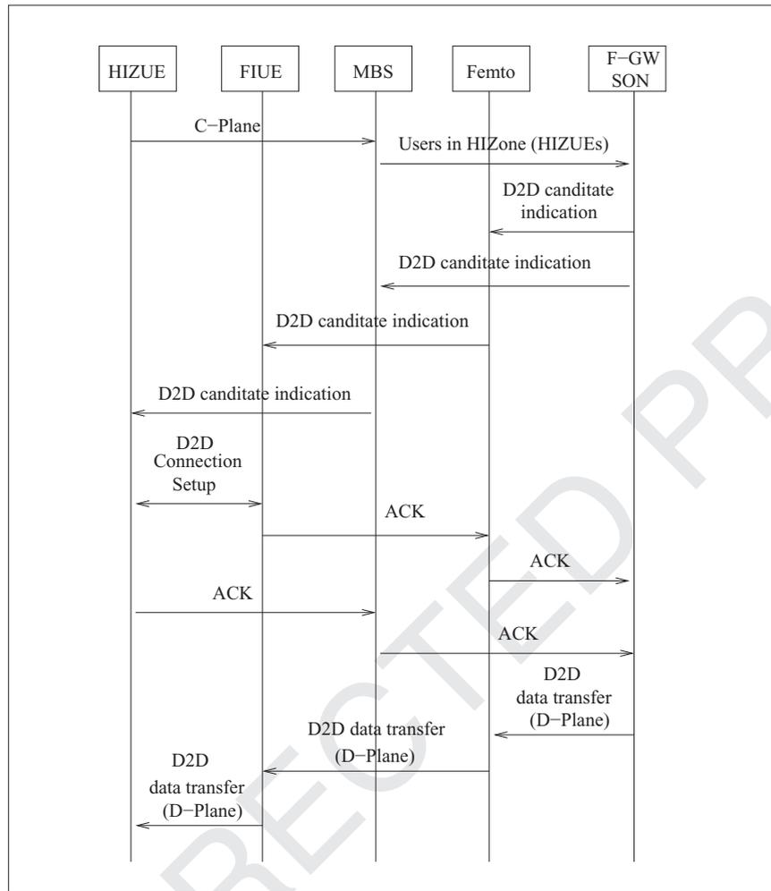
Fig. 4. Call flow diagram for D2D based communication in proposed HetNet system.
