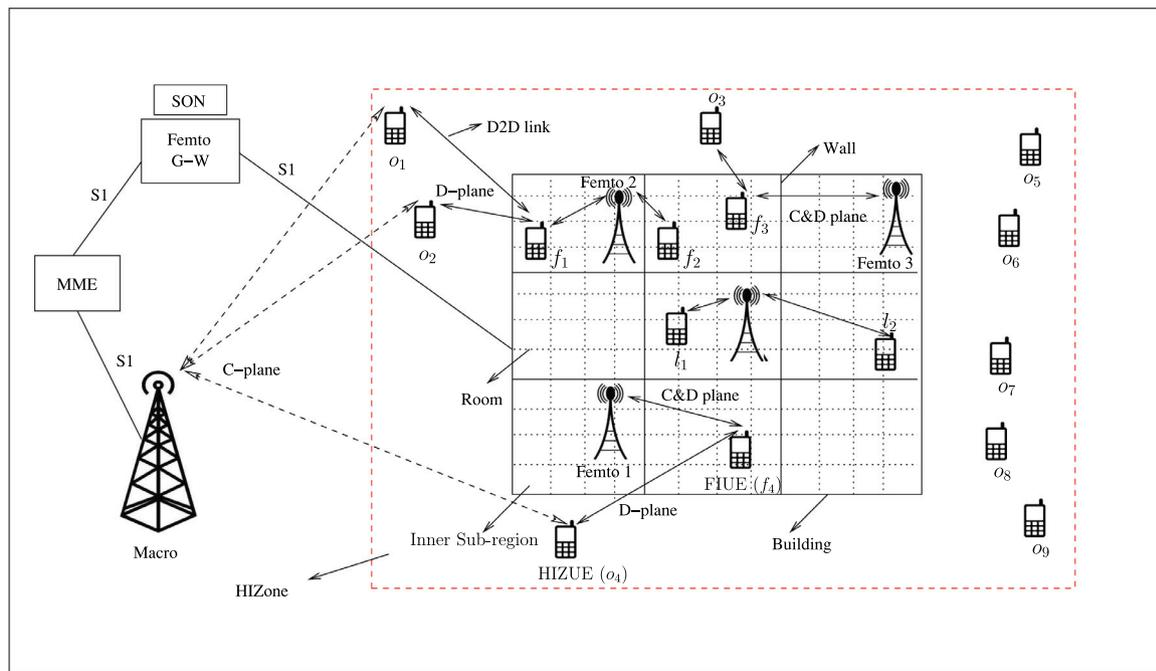
Fig. 3. Architecture of proposed HetNet system with D2D based relays.
