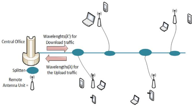
Fig. 1. A 60 GHz RoF network consisting of the optical domain and multiple antennas connected to the CO through a fiber bus.
