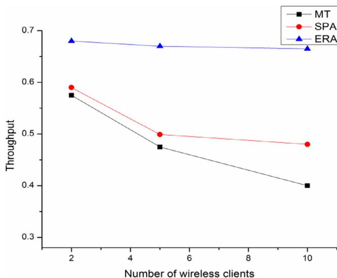
Fig. 21. Throughput results for different number of clients = 2, 5, 10 with network load 100%, 10 RAUs and 5 wavelengths.
