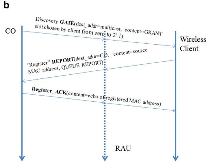
Fig. 3. (a) Recognizing wireless clients through the exponential back-off recognizing mechanism and traffic request collection procedure. (b) Wireless client's recognition and the structure of messages used for recognition.
