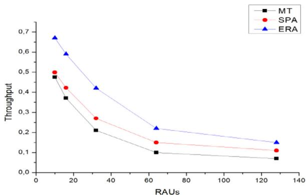
Fig. 19. Throughput results for different number of RAUs = 10, 16, 32, 64, 128, with network load 100%, 5 clients and 5 wavelengths.
