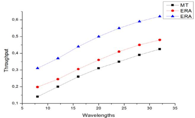
Fig. 17. Throughput results for different number of wavelengths  $w = 8, 12, 16, 20, 24, 28, 32$ , with network load 100%, 64 RAUs and 5 clients.
