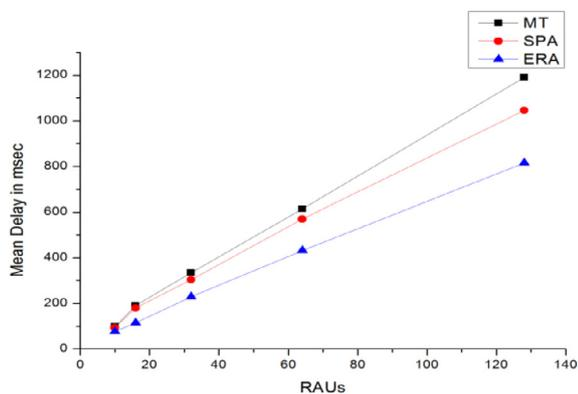
Fig. 18. Mean delay results for different number of RAUs = 10, 16, 32, 64, 128 with network load 100%, 5 clients and 5 wavelengths.
