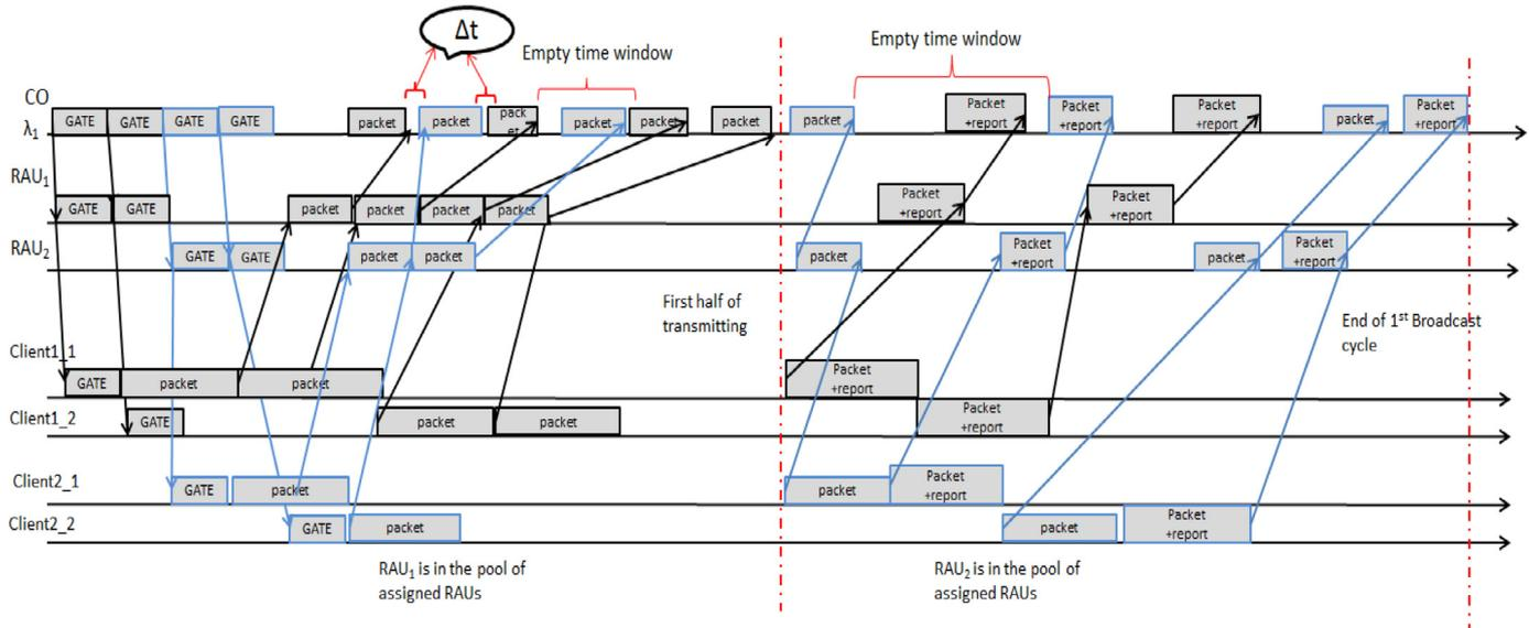
**Fig. 5.** The broadcast DATA period. This figure shows how the MPCP functions, specifically how a GATE message grants a transmission and the REPORT messages are collected in order to conduct a collision-free broadcast schedule. Additionally it shows the simultaneous use of wavelengths as aforementioned.
