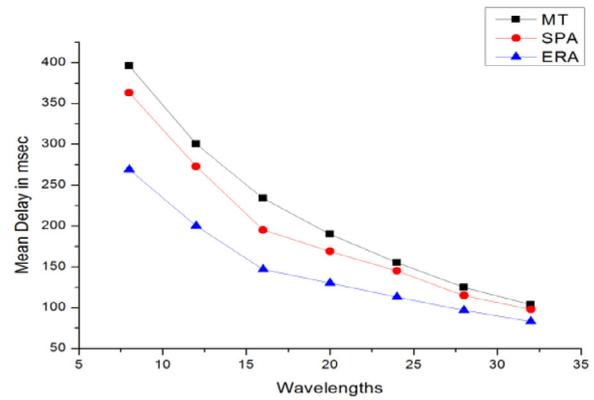
Fig. 16. Mean delay results for different number of wavelengths  $w = 8, 12, 16, 20, 24, 28, 32$ , with network load 100%, 64 RAUs and 5 clients.
