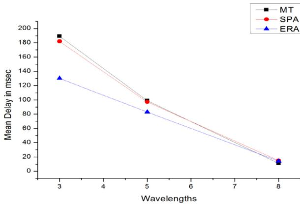
Fig. 14. Delay results for different number of wavelengths, with network load 100%, 10 RAUs and 5 clients.
