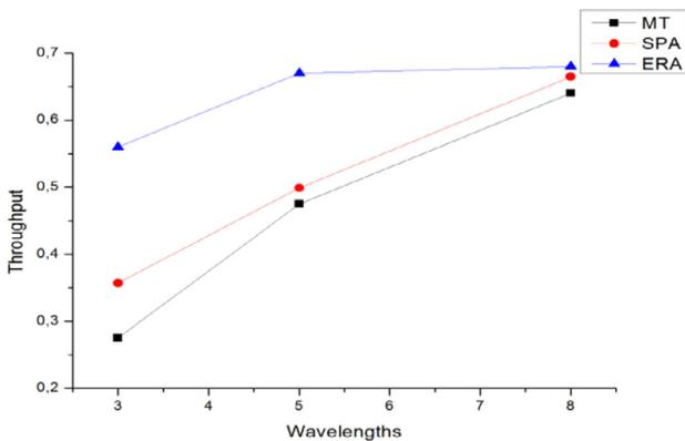
Fig. 15. Throughput results for different number of wavelengths, with network load 100%, 10 RAUs and 5 clients.
