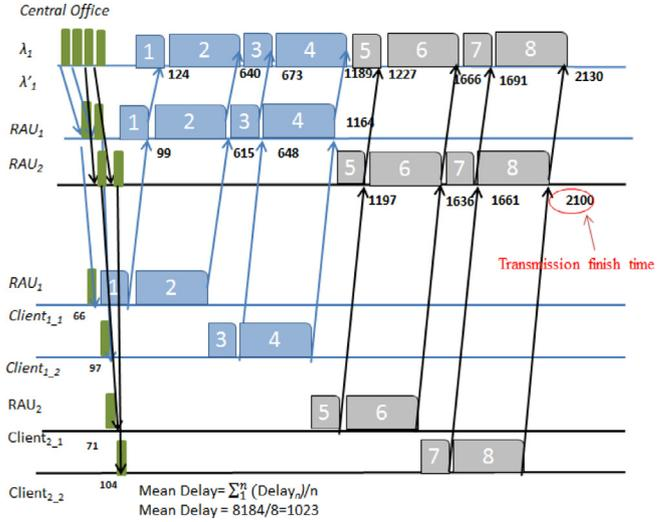
Fig. 7. MT-MAC protocol's broadcast schedule. The numbers in the figure show us the time that a packet is completely received from RAUs and subsequently from the CO.
