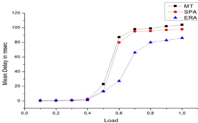
**Fig. 10.** Mean packet delay as a function of network load for 64 RAUs and 5 clients under each RAU, and  $w = 32$  number of wavelengths.
