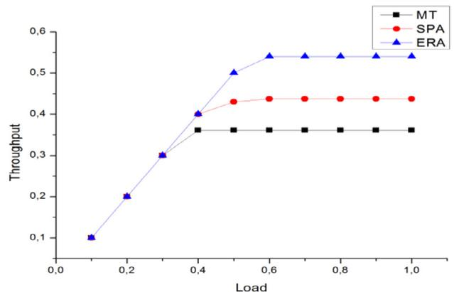
**Fig. 13.** Network throughput as a function of network load for 128 RAUs and 5 clients under each RAU and  $w = 64$  number of wavelengths.
