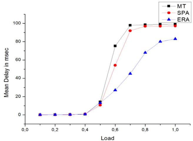
Fig. 8. Mean packet delay as a function of network load for 10 RAUs and 5 clients under each RAU, and  $w = 5$  number of wavelengths.
