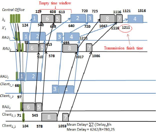
Fig. 6. ERA protocol's broadcast schedule. The numbers in the figure show us the time that a packet starts being received and when it is completely received from RAUs and afterwards from the CO.
