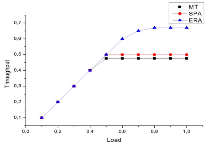
Fig. 9. Network throughput as a function of network load for 10 RAUs and 5 clients under each RAU and  $w = 5$  number of wavelengths.
