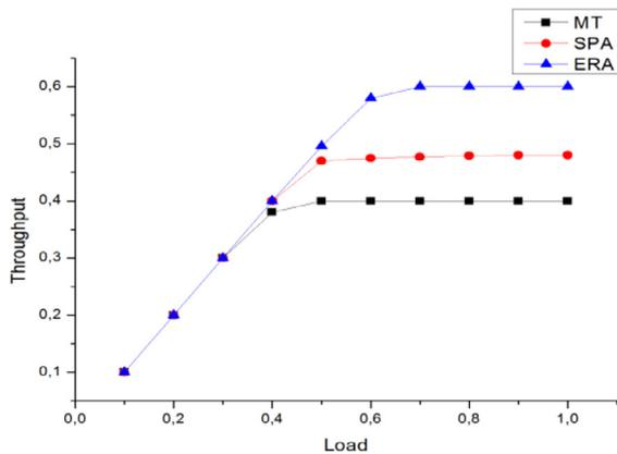
**Fig. 11.** Network throughput as a function of network load for 64 RAUs and 5 clients under each RAU and  $w = 32$  number of wavelengths.
