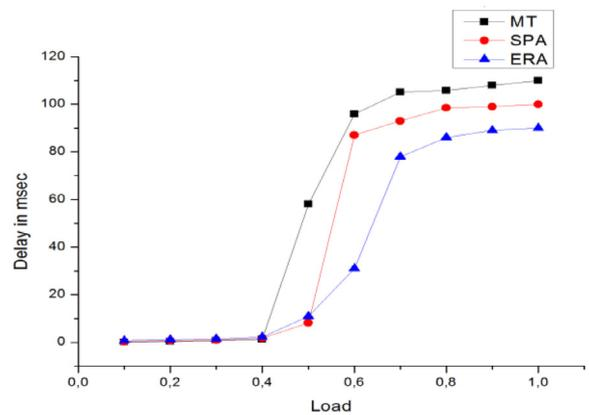
**Fig. 12.** Mean packet delay as a function of network load for 128 RAUs and 5 clients under each RAU, and  $w = 64$  number of wavelengths.
