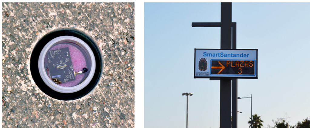
Fig. 1. Parking sensors buried under the road surface and Notification Displays to show free parking spots.
