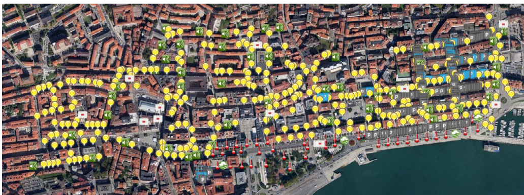
Fig. 2. Outdoor deployment of 400 parking sensors and 10 notification panels at the city of Santander.
