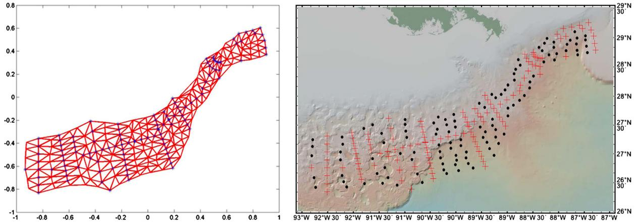
**Fig. 11.** A triangulation with rescaled measurement locations (in blue dots; left, using scaled coordinates) and an image of the seafloor topography (right, with longitudes and latitudes) with measurement locations (in red crosses) and added vertices (black dots). (For interpretation of the references to color in this figure legend, the reader is referred to the web version of this article.)
