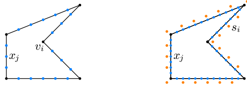
Fig. 3. Nodes used by BEM (left) and nodes and sites used by MFS (right).
