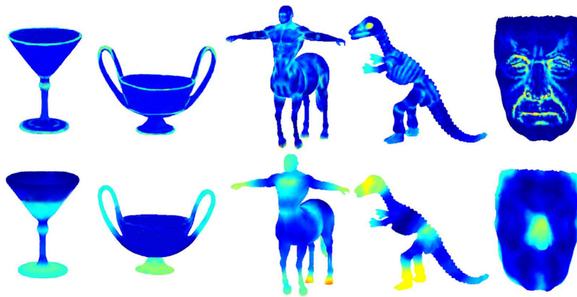
Fig. 6. Mesh saliency results on various models. The top row shows local feature saliency (from left to right r = 3, 3, 4, 4, 3 , respectively), and the bottom row shows global structure saliency (from left to right r = 24, 23, 30, 25, 24 , respectively).
