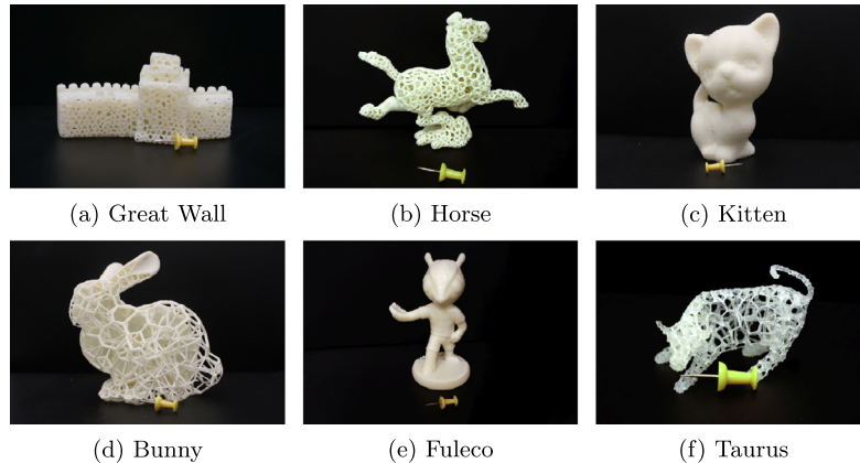
Fig. 12. Printed objects. The models in (a), (c), (d) and (e) are printed by uPrint SE Plus printer; model (b) is printed by uPrint SE printer and (f) by Projet® 3500 HDMax.
