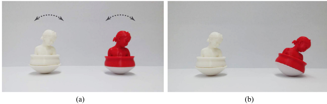
Fig. 8. Examples of girls. (a) is the balancing state. \mathcal{U} use the same model. The white one is optimized using P and the red one is optimized without using P . The optimized results are a = 0.0234 , r = 25.7556 for the left one and a = 0.0237 , r = 23.9305 for the right one consequently. After pushing them in (a), the white one is more likely to regain its balancing state, while the red one is not, as shown in (b). (For interpretation of the references to color in this figure legend, the reader is referred to the web version of this article.)
