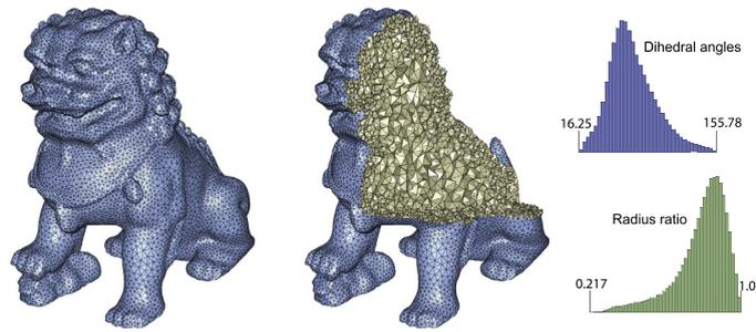
**Fig. 1.** An example of our tetrahedral meshing result on the Lion model (input 100K triangles). Left and middle are the meshing result (55K vertices and 300K cells) and a cutaway view, respectively. Right are the dihedral angle and radius ratio distributions.
