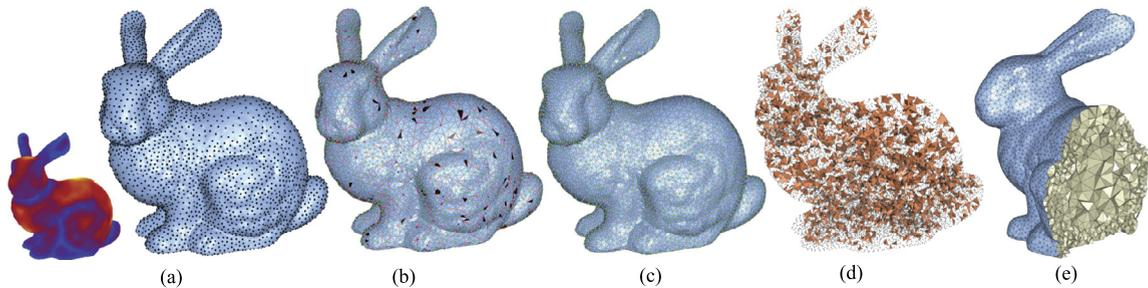
**Fig. 3.** Overview of our algorithm. Given the input boundary mesh, we first generate surface samples (a) and extract a surface mesh (b). We optimize the boundary remeshing to improve its quality (c). After the boundary optimization, we perform volume sampling while showing slivers (d). Then we optimize the dihedral angles to remove these slivers. (e) is a cutaway view of the final mesh.
