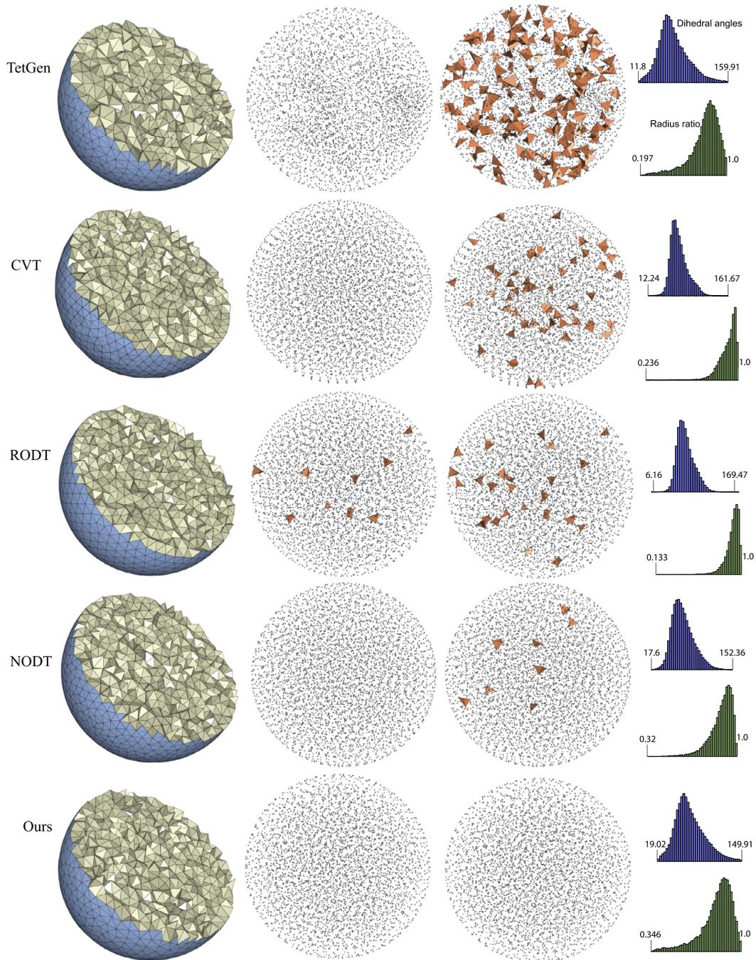
**Fig. 11.** Comparison of our uniform tetrahedral mesh with those produced by other algorithms. For each row, from left to right we show the cutaway view of meshing result, slivers with dihedral angles smaller than  $10^\circ$  and  $18^\circ$ , and distributions of dihedral angles (blue) and radius ratios (green). (For interpretation of the references to color in this figure legend, the reader is referred to the web version of this article.)
