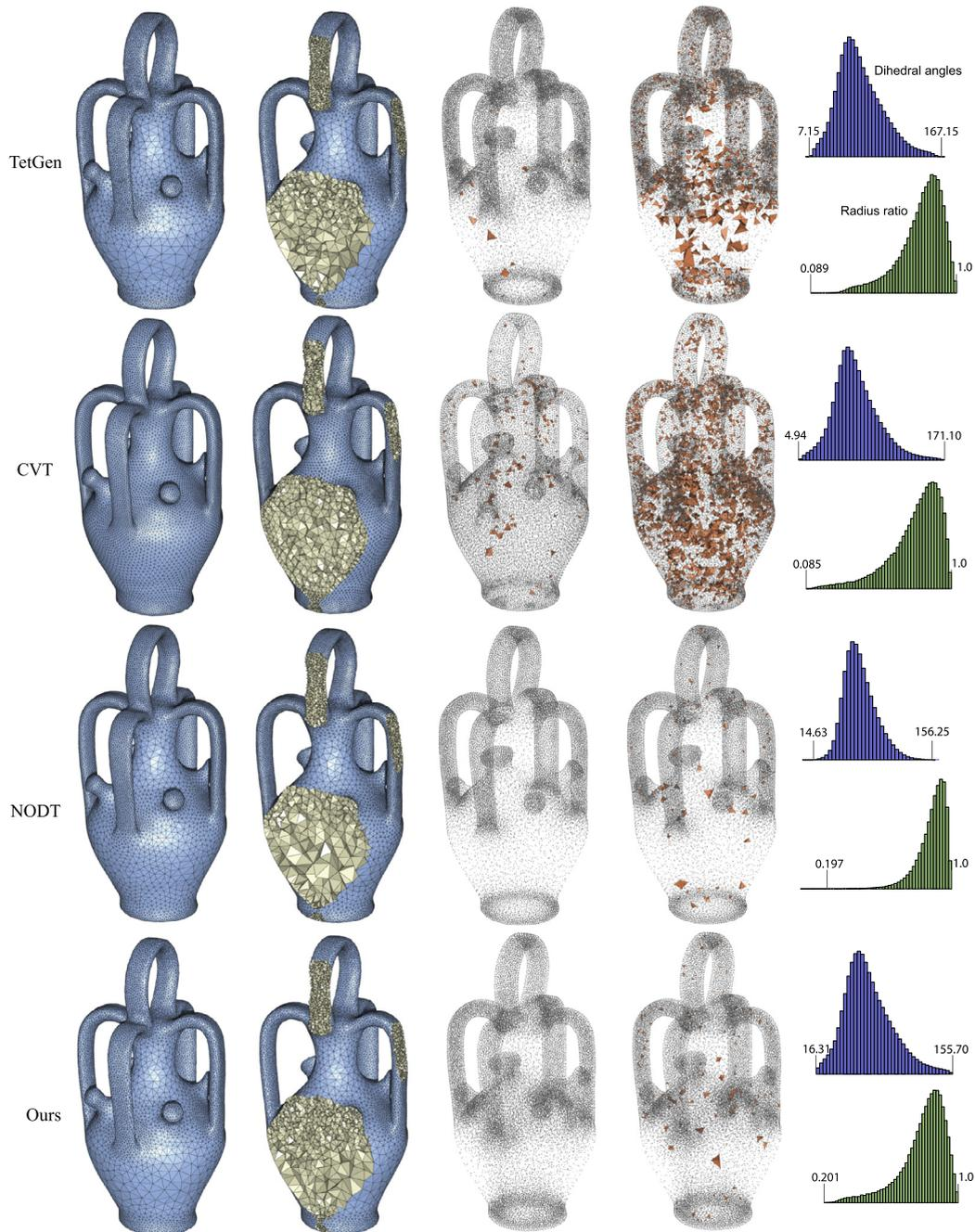
**Fig. 10.** Comparison between different algorithms in generating a graded tetrahedral mesh. For each row, from left to right we show the meshing result, its cutaway view, slivers with dihedral angles smaller than  $10^\circ$  and  $18^\circ$ , and distributions of dihedral angles (blue) and radius ratios (green). (For interpretation of the references to color in this figure legend, the reader is referred to the web version of this article.)
