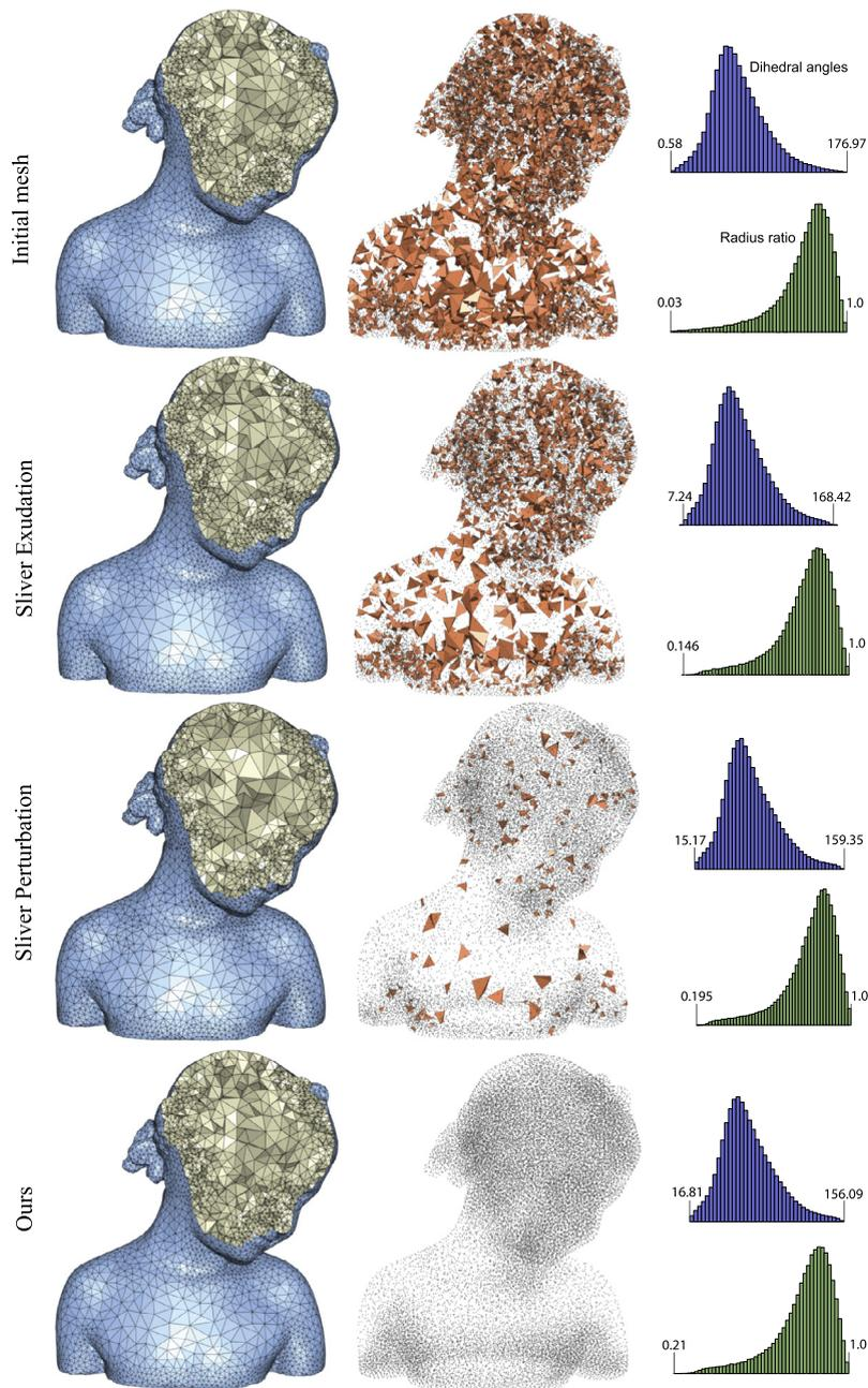
**Fig. 13.** Comparison with sliver exudation (Cheng et al., 2000) and sliver perturbation (Tournois et al., 2009) on the Bimba model. Left: cutaway view of the initial mesh and the optimized mesh; middle: sliver tetrahedra for a dihedral angle of 17 degrees; right: dihedral angle distributions (blue), and radius ratio distributions (green). (For interpretation of the references to color in this figure legend, the reader is referred to the web version of this article.)
