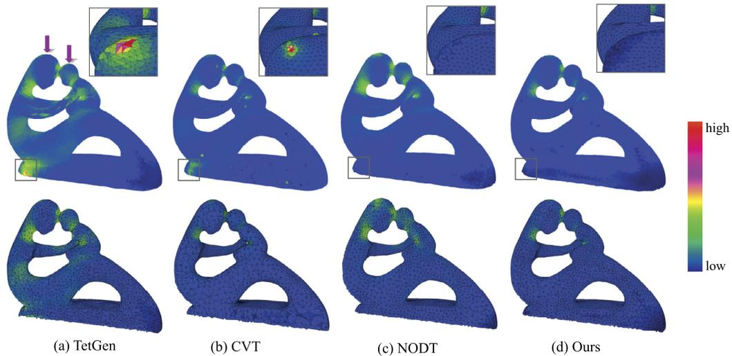
**Fig. 12.** Structural analysis with the same force settings (arrows in (a)). The top row shows the stress map with color coding (zoom-in figures show a slightly different view), and the bottom row shows the interior structure.
