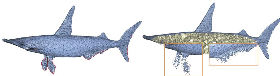
**Fig. 14.** Our algorithm cannot guarantee a pleasant result when the minimal radius is larger than the local feature size of the domain. Left: surface remeshing after the boundary sampling stage. The non-manifold edges are shown in red. Right: tetrahedral meshing result with two zoom-in views. (For interpretation of the references to color in this figure legend, the reader is referred to the web version of this article.)
