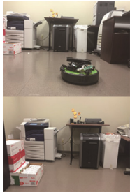
Fig. 10. (Left): Diagram of system architecture. The Raspberry Pi acts as a hub and controller for the rest of the devices in the system. (Right): Our iRobot carrying a Raspberry Pi and a Kinect.
