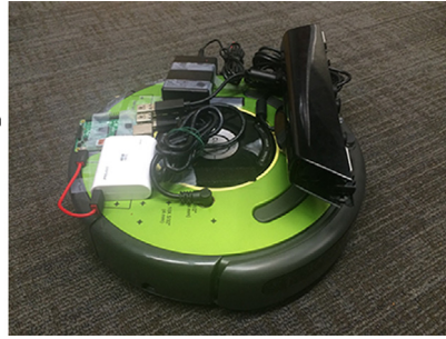
Fig. 10. (Left): Diagram of system architecture. The Raspberry Pi acts as a hub and controller for the rest of the devices in the system. (Right): Our iRobot carrying a Raspberry Pi and a Kinect.
