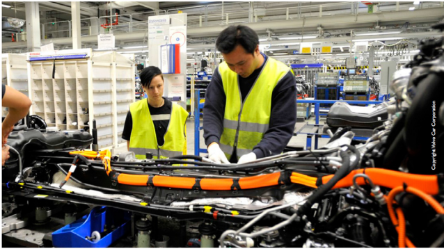
Fig. 1. Assembly of a high-voltage power cable in a hybrid car. © 2014, Volvo Car Corporation.
