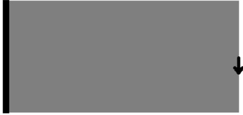
Fig. 6. The cantilever structure problem (100 \* 50).
