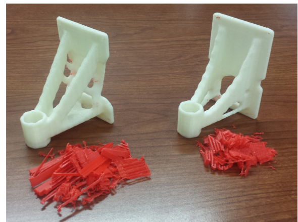
Fig. 25. Printed mount bracket and the required support structures at 0.7 volume fraction.
