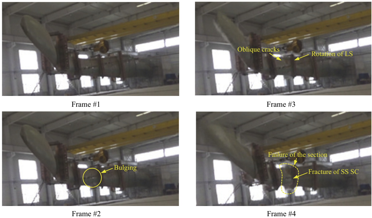
(b) Collapse process captured by camera #2
