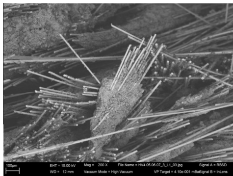
(a) SEM image of a fracture area of an SMC sample depicting glass fiber bundles and the surrounding matrix material
