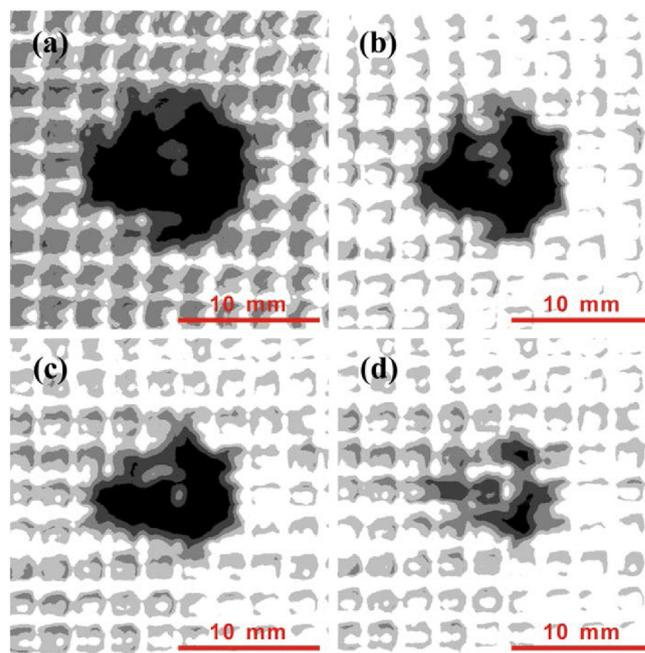
**Fig. 7.** Ultrasonic T-scan images of the indentation damaged composite laminates with the embedded healing agent-loaded PP tubes (tube spacing: 750  $\mu\text{m}$ ; foaming agent content: 3 parts; foaming condition: 70  $^{\circ}\text{C}$ , 8 h; healing temperature: 25  $^{\circ}\text{C}$ ). Time of healing: (a) 2.0 h, (b) 12.0 h, (c) 24.0 h, and (d) 36.0 h. Damage area: (a) 74.4  $\text{mm}^2$ , (b) 53.8  $\text{mm}^2$ , (c) 39.1  $\text{mm}^2$ , and (d) 5.4  $\text{mm}^2$ .
