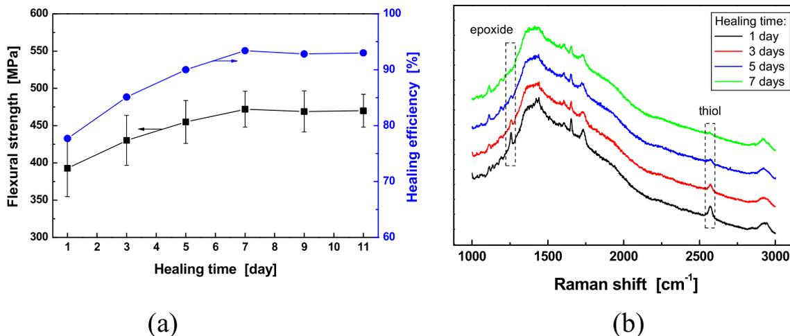
**Fig. 6.** (a) Effect of healing time on flexural strength and healing efficiency of the healed composite laminates with the embedded healing agent-loaded PP tubes (tube spacing: 750  $\mu\text{m}$ ; foaming agent content: 3 parts; foaming condition: 70  $^{\circ}\text{C}$ , 8 h; healing condition: 25  $^{\circ}\text{C}$ ). (b) In-situ confocal Raman microscopy spectra collected from the fractured surface of the above composites.
