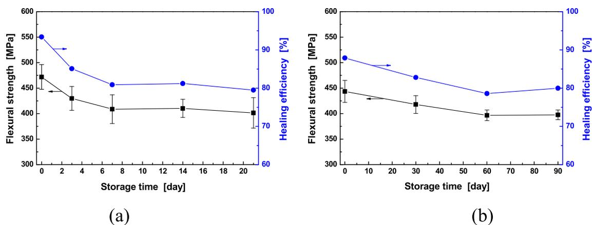
**Fig. 8.** Effect of room temperature storage time on flexural strength and healing efficiency of the healed composite laminates with the embedded healing agent-loaded PP tubes (foaming agent content: 3 parts). Healing condition: 25 °C, 7 days. Foaming condition: (a) 70 °C, 8 h; (b) 70 °C, 4 h.
