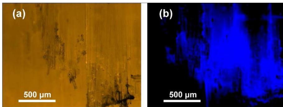
**Fig. 5.** Fluorescent microscopy photos of back face of the composite laminates with the healing agent-loaded PP tubes (tube spacing: 750 μm; foaming agent content: 3 parts; foaming condition: 70 °C, 8 h). The composite was damaged by indentation. The photos were taken under the lights of (a) 525 nm and (b) 365 nm, respectively. Information of the fluorescent penetrant refers to Fig. 3(b).
