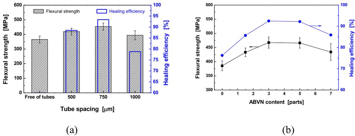
**Fig. 4.** Effect of (a) tube spacing and (b) foaming agent content on flexural strength and healing efficiency of the damaged and healed composite laminates with the embedded healing agent-loaded PP tubes. Flexural strength of the damaged laminates without PP tubes is shown in (a) as reference. Tube spacing for (b): 750 μm. Foaming agent content: 3 parts; foaming condition: 70 °C, 8 h; healing condition: 25 °C, 7 days.
