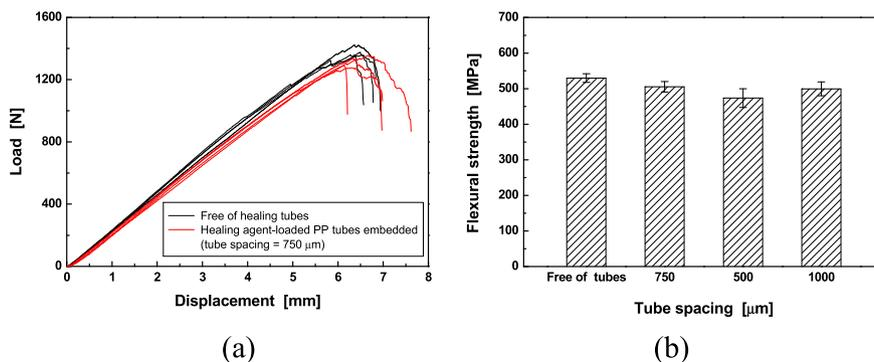
**Fig. 2.** (a) Load-displacement curves and (b) flexural strengths of the composite laminates with and without the healing agent-loaded PP tubes measured by four-point bend tests.
