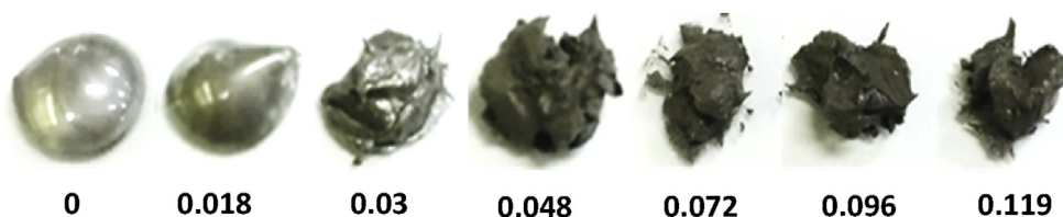
Fig. 3. Macroscopic observation of the transition from fluid-like behavior to solid-like behavior with different \rho .
