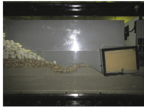
Fig. 12. Final configuration of the collapsed caisson due to coupled tsunami overflow and seepage.
