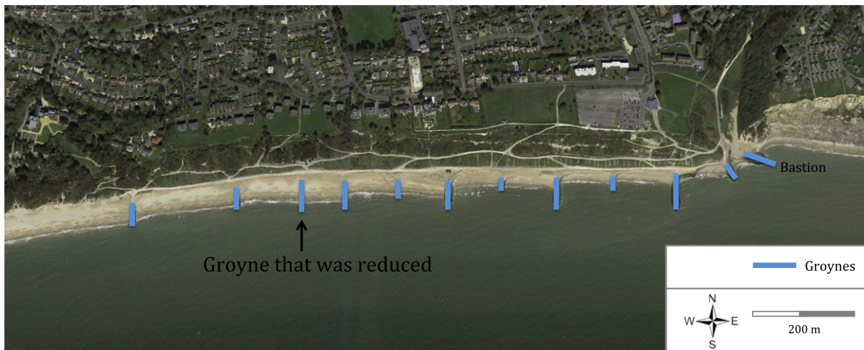
Fig. 2.2. Image of the groyne system constructed at Highcliffe within Christchurch bay. Image shows the eleven rock groynes and a bastion of varying long and short lengths, and highlights the study groyne that was reduced. Image adapted from Imagery ©2016 Google, TerraMetrics, Map data ©2016 Google.
