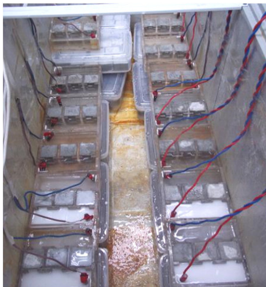
Fig. 3. The test setup of TSA formation via the action of electrical pulses in a refrigerating cabinet.
