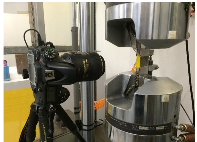
Fig. 3. A camera is placed in front of the specimen to capture crack patterns.
