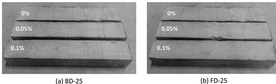
Fig. 9. Crack reduction with increasing fibre dosage in M4.
