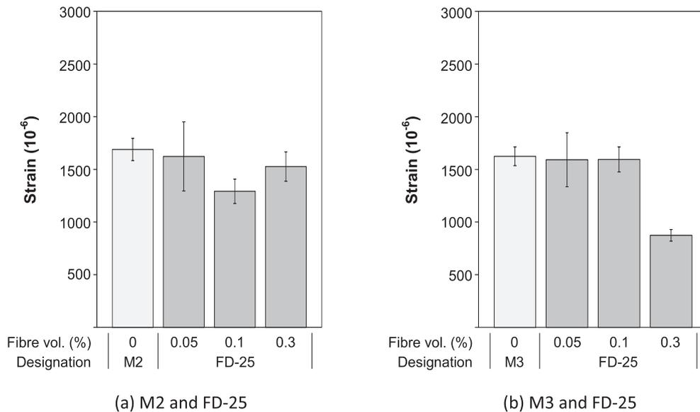
Fig. 8. Mean strain values measured after 4 h.
