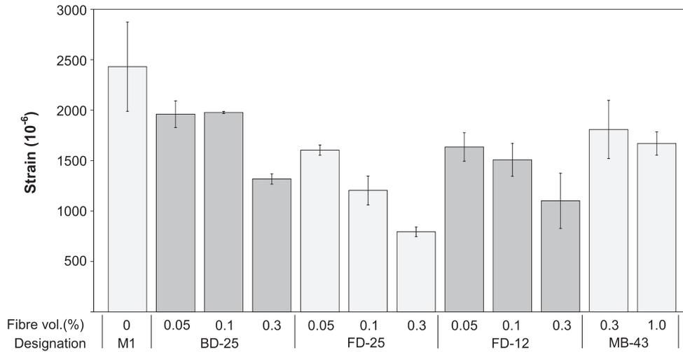
Fig. 6. Mean strain values measured after 4 h in control mix (M1).
