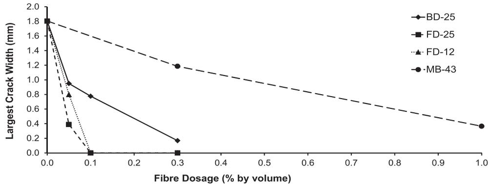
Fig. 11. Effect of fibres on crack width on specimen surface in M4.
