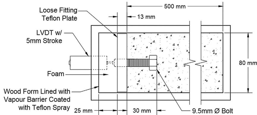
Fig. 2. Free plastic shrinkage test setup.
