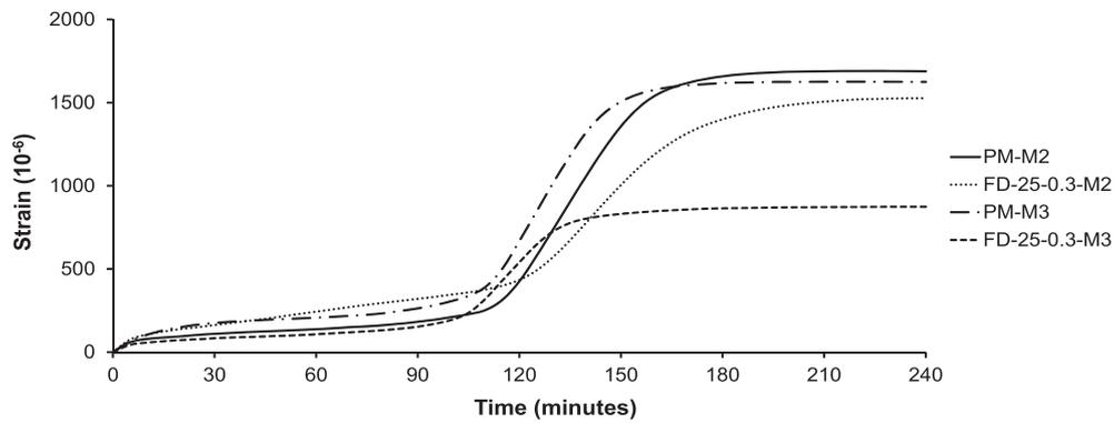
Fig. 7. Comparison between reduced w/c ratio mix (M2) and concrete mix (M3).
