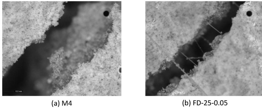
Fig. 12. Crack development without fibre (a) and with fibre (b).
