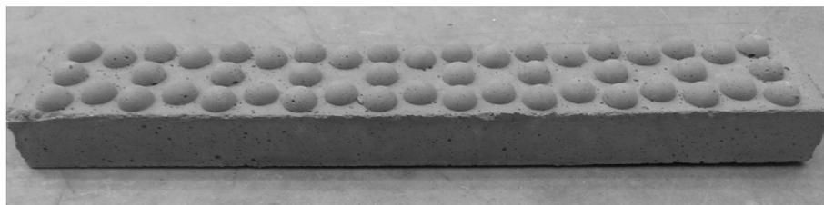
(a) High-strength concrete restraint element
