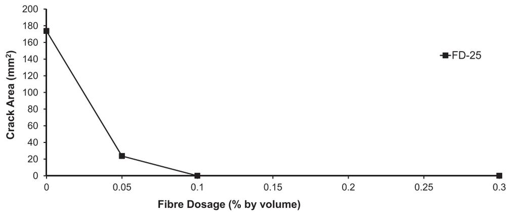
Fig. 13. Effect of FD-25 on crack area in low w/c ratio mix M5.
