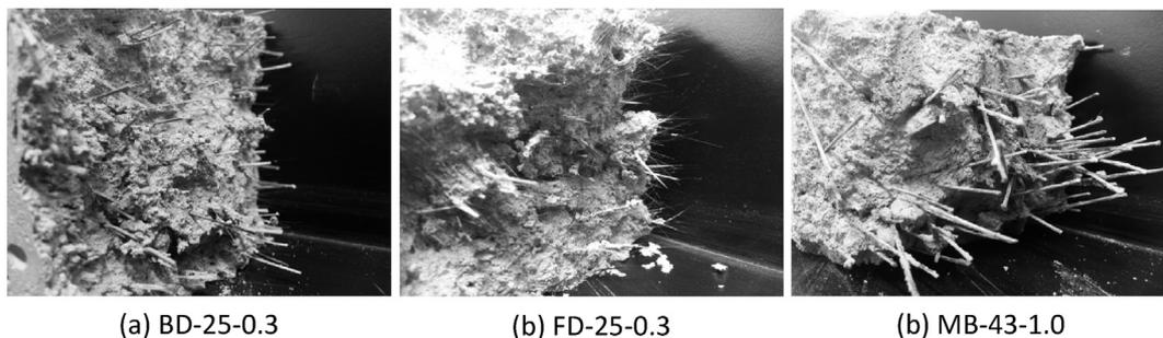
**Fig. 4.** Difference in dispersion of fibres used in this study.
