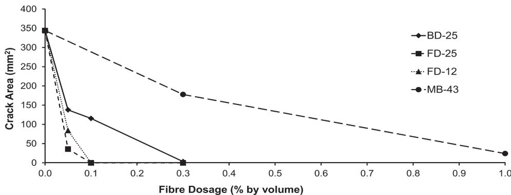
Fig. 10. Effect of fibres on total crack area on specimen surface in M4.
