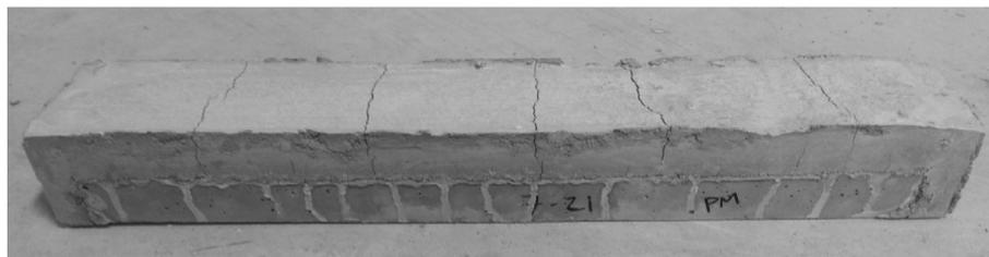
(b) 35 mm thick mortar overlay after four hours in environmental chamber
