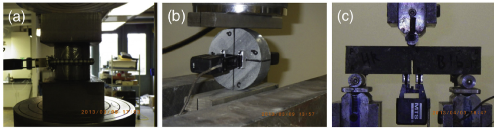
Fig. 2. UHPC experiment setup: (a) cylinder compression, (b) splitting, (c) beam 3-point-bending.
