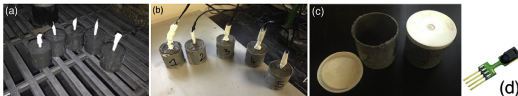
Fig. 3. Relative humidity measurement: (a) specimens curing, (b) measurement setup, (c) plastic molds, (d) RH&T sensor.
