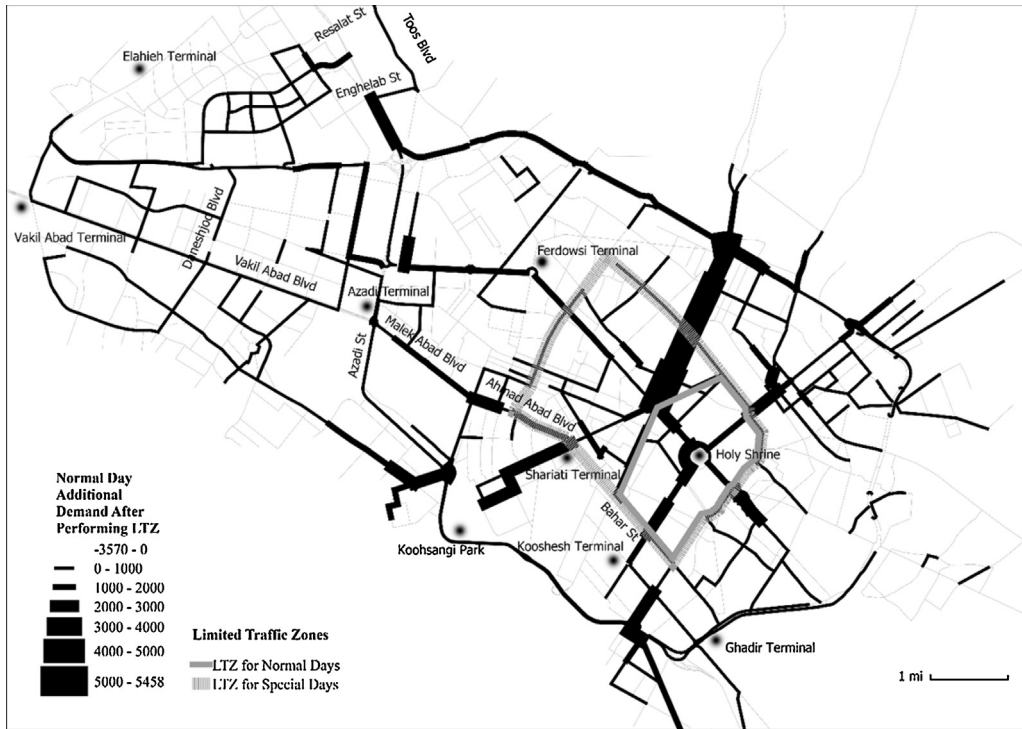
Fig. 3. Additional demand of bus transit system in normal days after performing LTZ, \delta^{a,n} .
