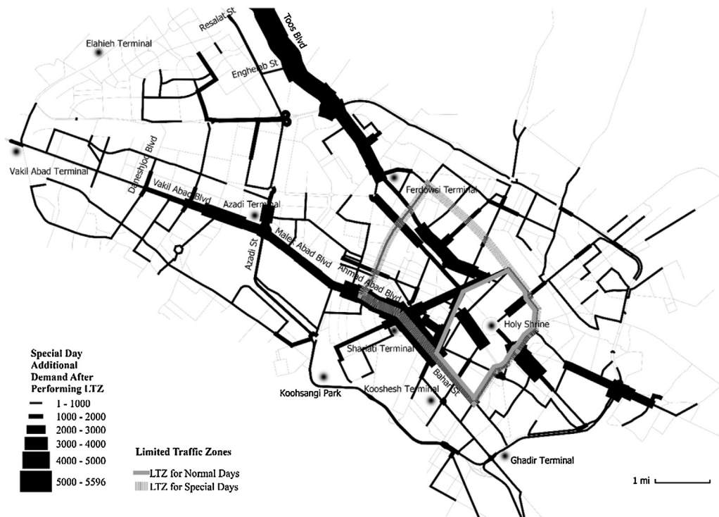
Fig. 4. Additional demand of bus transit system in special days after performing LTZ, \delta^{a,s} .
