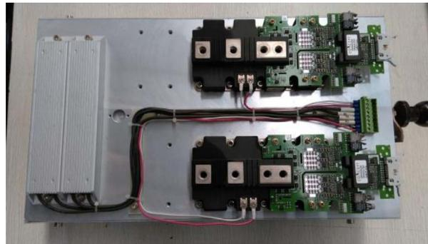
(b) Material object of power module block
