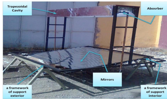
Fig. 1. Scheme of the experimental device.
