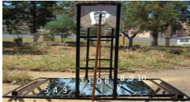
Fig. 3. The configuration of mirrors at 12:00.
