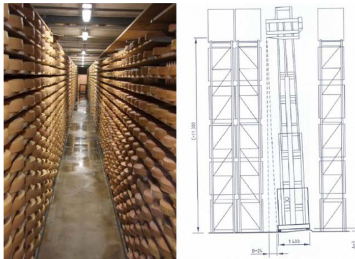
Fig. 3. The levelness of industrial floor can influence the height storage capacity.
