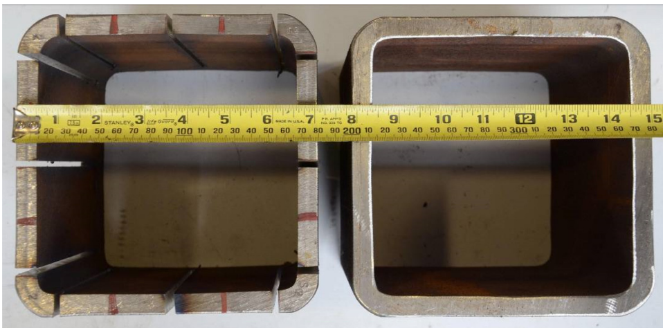
Fig. 13. Sectioning test results of the hot-formed SHS.
