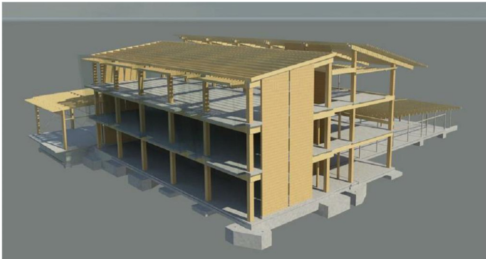
Fig. 1. 3D view of the NMIT Arts and Media Building Structure.
