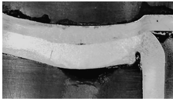
Fig. 3. Macrographic view of welded joint cross-section.
