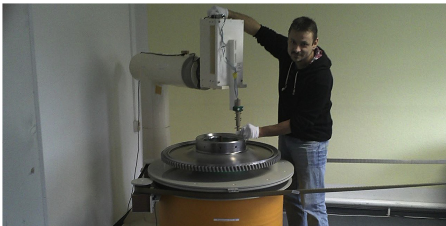
Fig. 2. Measurement setup for the analysis of a rotating aeroengine turbine disk with a fluxgate magnetometer [8].
