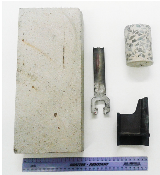
Fig. 1. Photo of the samples with a 30 cm scale bar at the bottom – on the left is a concrete block with metal fiber reinforcement, in the middle is a steel turbine blade, on the top right is a concrete cylinder and on the bottom right is a titanium investment casting.
