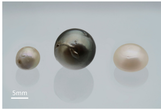
Fig. 1. (From left to right): saltwater natural pearl (NP-2f), beaded saltwater cultured pearl (CP-2f) and beadless freshwater cultured pearl (CP-1b).
