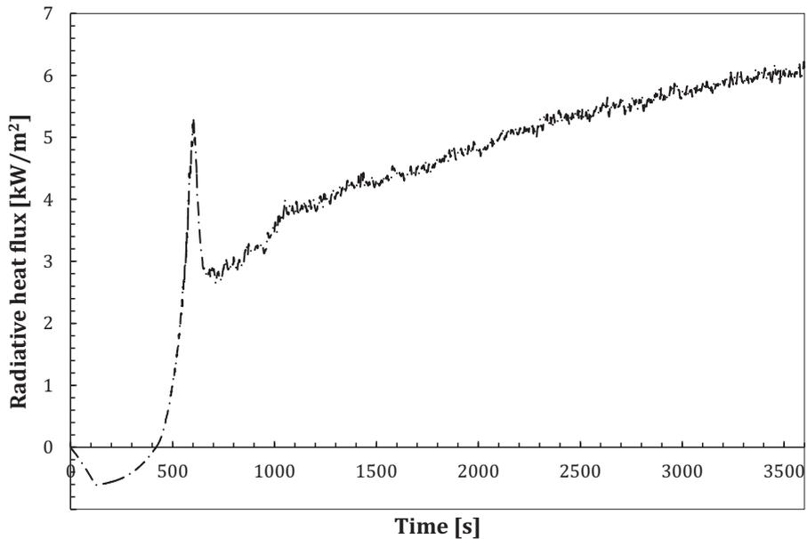
Fig. 5. Radiative feedback to the fuel surface as a function of time using insulated walls, one door opening and a growth rate of  $0.003 \text{ kW/s}^2$ .
