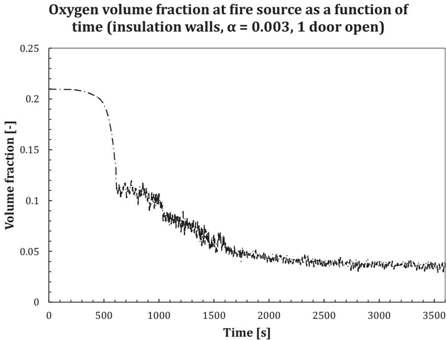
Fig. 4. Oxygen volume fraction close to the fire source as a function of time using insulated walls, one door opening and a growth rate of  $0.003 \text{ kW/s}^2$ .
