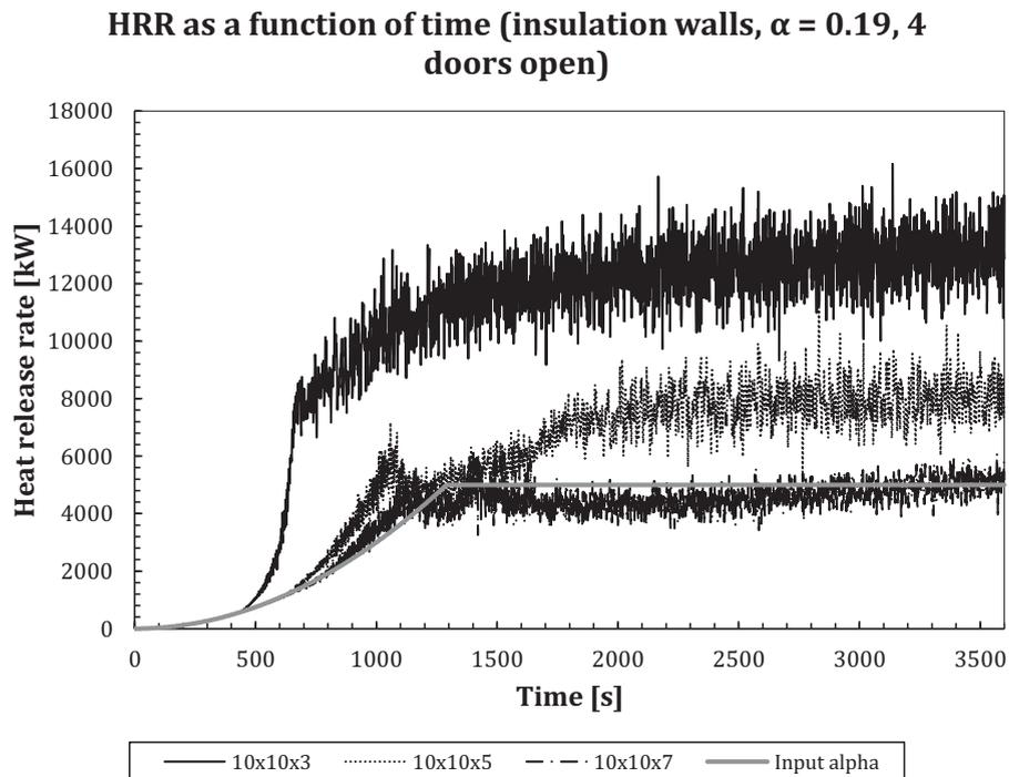
**Fig. 10.** Heat release rate as a function of time using different ceiling heights, four door openings and a growth rate of  $0.003 \text{ kW/s}^2$ .
