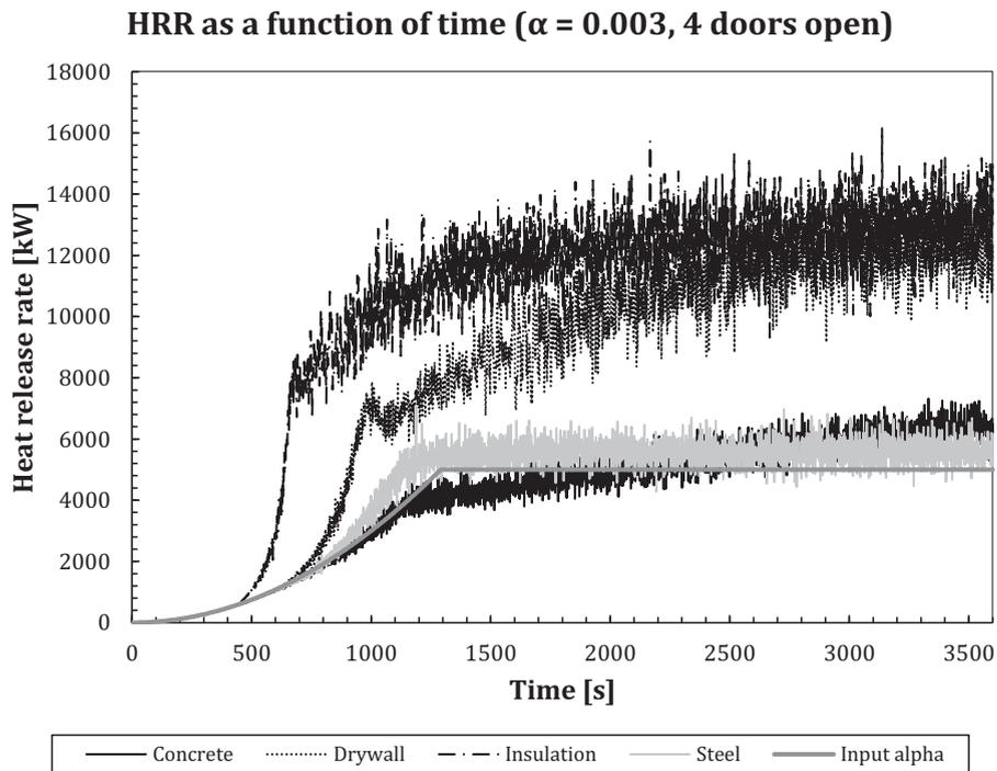
**Fig. 6.** Heat release rate as a function of time using different building materials, four door openings and a growth rate of  $0.003 \text{ kW/s}^2$ .**Table 12**
