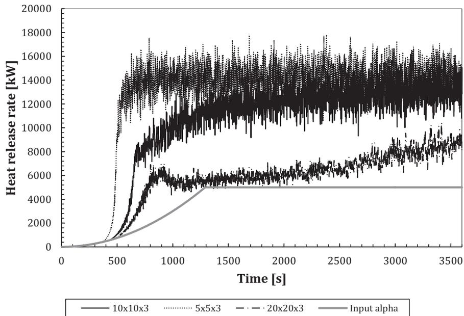
Fig. 8. Heat release rate as a function of time using different room floor areas, four door openings and a growth rate of 0.003 kW/s<sup>2</sup>.
