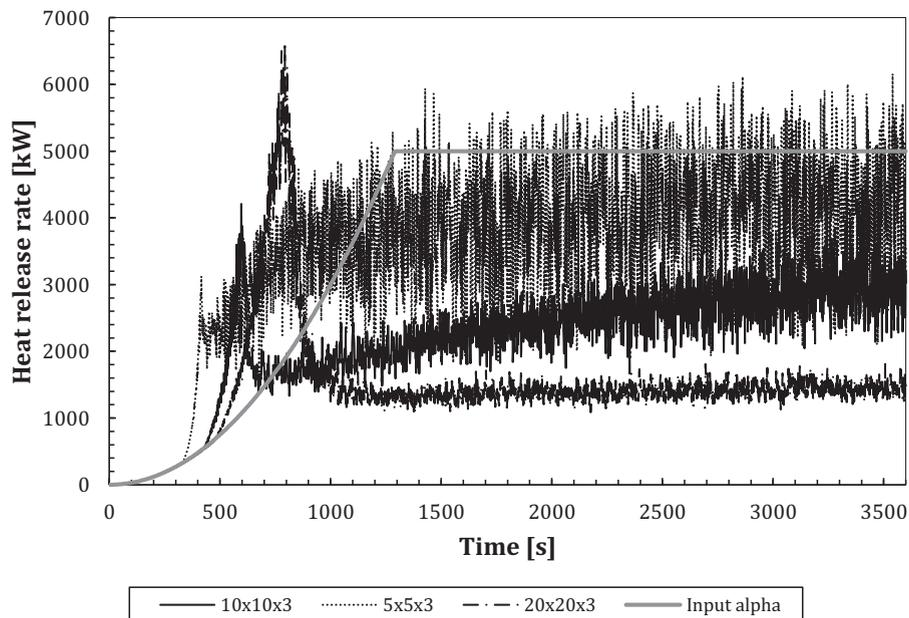
**Fig. 7.** Heat release rate as a function of time using different room floor areas, one door opening and a growth rate of 0.003 kW/s<sup>2</sup>.
