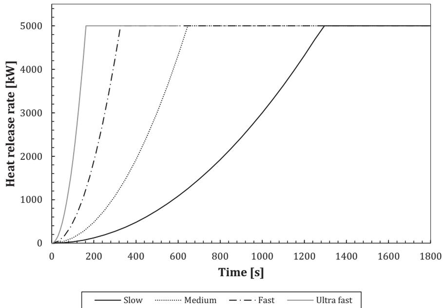
Fig. 1. Visual representation of the different standard growth rates according to NFPA 204M [5].
