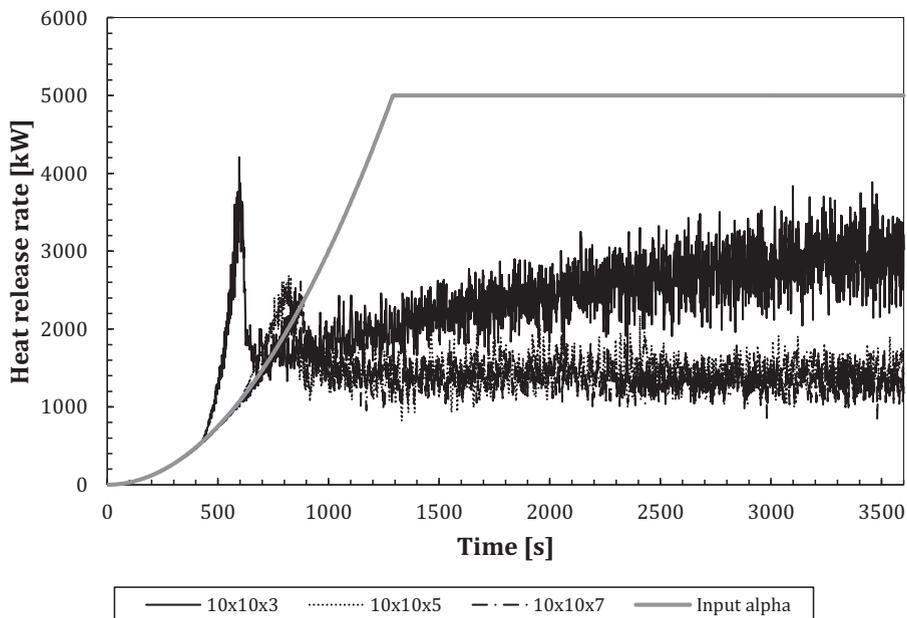
**Fig. 9.** Heat release rate as a function of time using different ceiling heights, one door opening and a growth rate of 0.003 kW/s<sup>2</sup>.
