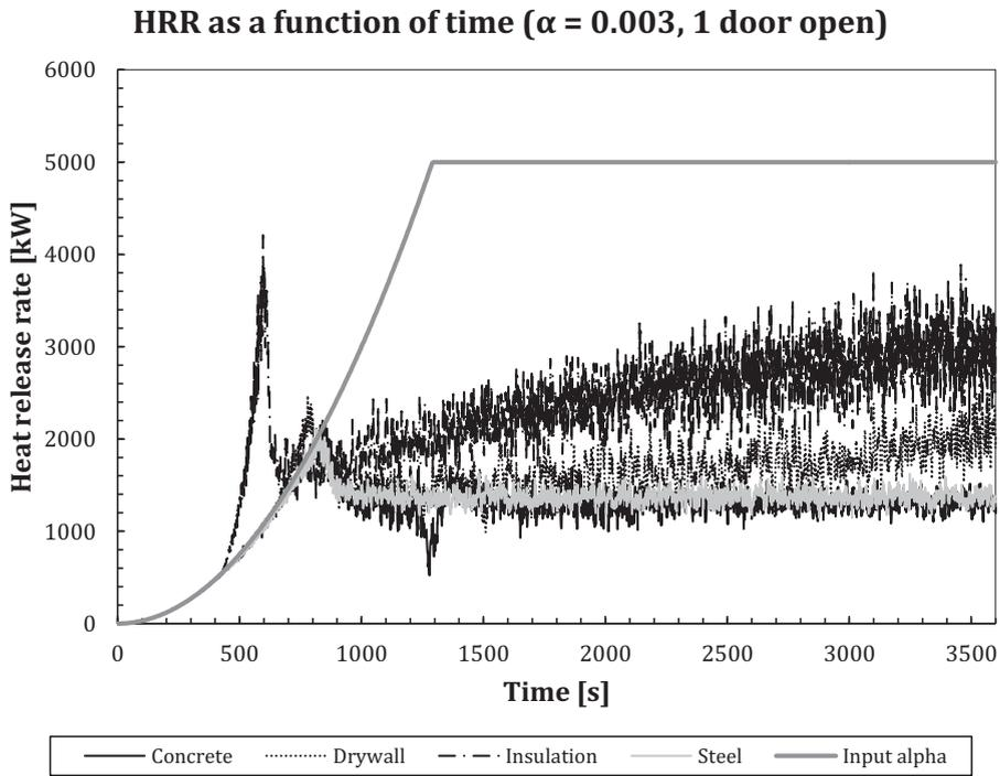
Fig. 3. Heat release rate as a function of time using different building materials, one door opening and a growth rate of  $0.003 \text{ kW/s}^2$ .
