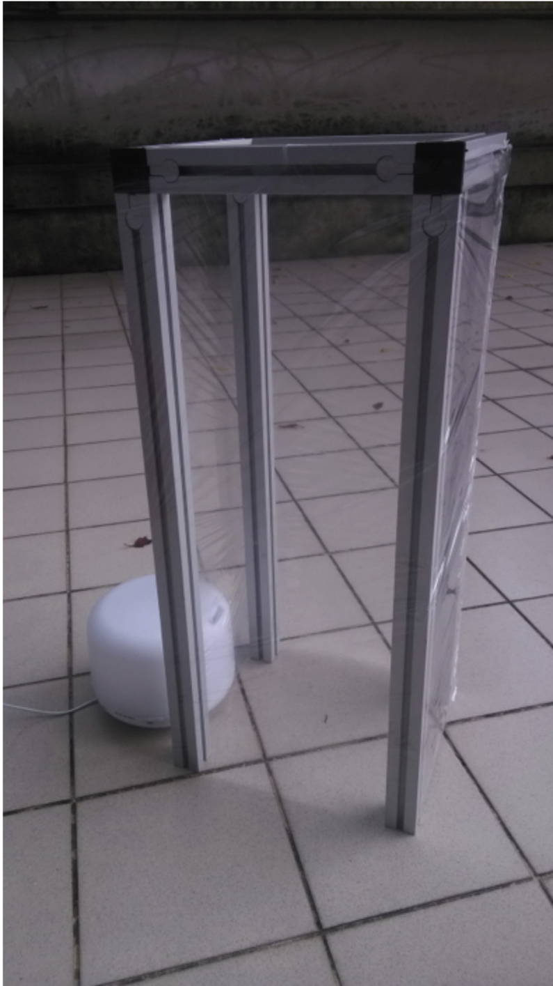
Fig. 2. Restricted airflow chamber with adjacent MUJI nebulizer.
