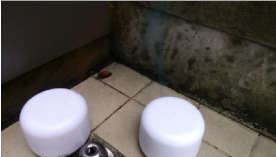
Fig. 5. MUJI nebulizers dispensing red (left) and blue (right) mist outdoors in a slight breeze. (For interpretation of the references to colour in this figure legend, the reader is referred to the web version of this article.)
