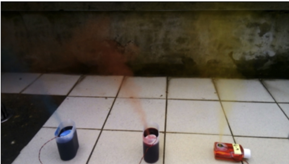
Fig. 6. Mesh nebulizers dispensing blue, red, and yellow mist outdoors with a slight breeze present. (For interpretation of the references to colour in this figure legend, the reader is referred to the web version of this article.)
