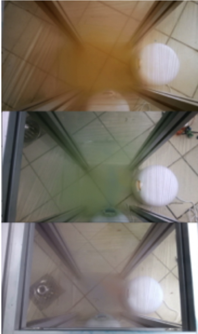
Fig. 4. Combination of two nebulizers dispensing different colored mists after 25 s.
