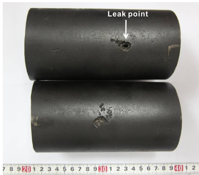
Fig. 1. Examples of the failed pipes. The leak point is indicated by the white arrow.
