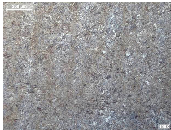
Fig. 4. Microstructure of the connecting rod material.
