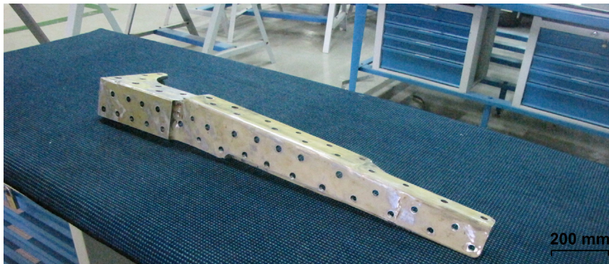
Fig. 1. Image of cracked internal angel after removing from A/C.
