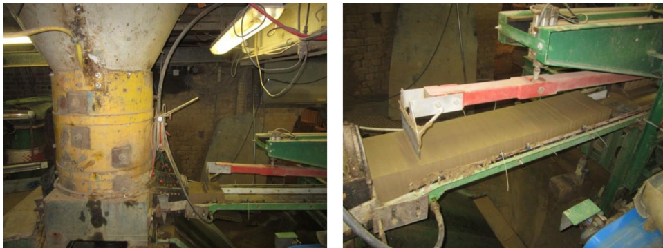
Fig. 3. Extrusion of unfired clay bricks.
