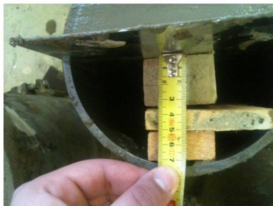
Fig. 2. Aluminum plate inserted at mold centerline to create CJ.
