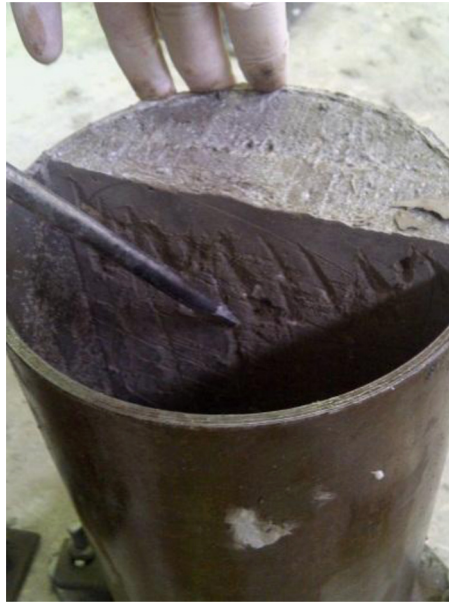
Fig. 4. Roughening the construction joint face.
