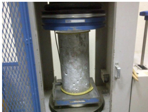
Fig. 5. UTM testing of cylinder.
