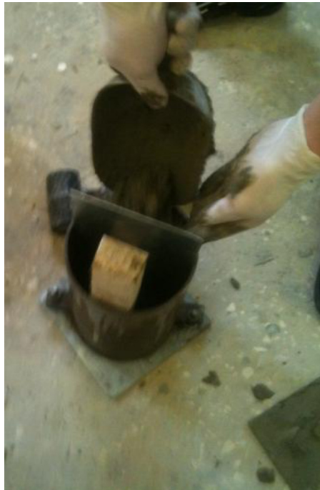
Fig. 3. Pouring the non-monolithic cylinders.
