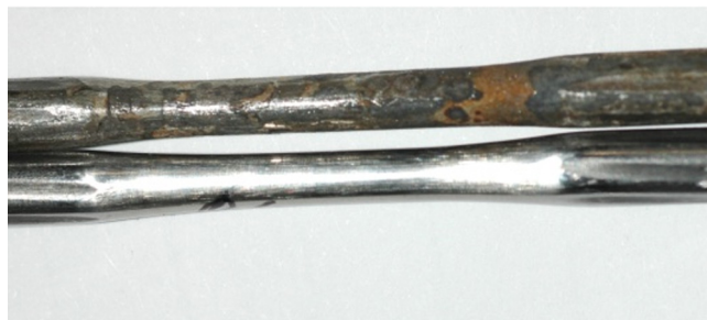
Fig. 7. Two specimens with and without the effect of corrosion in the tap water.
