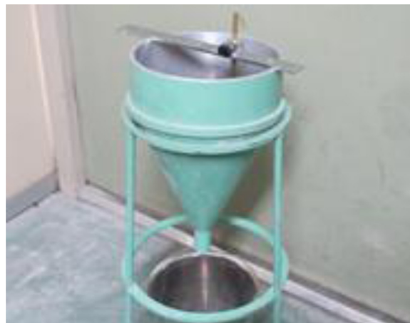
Fig. 1. P-type funnel used for a fluidity test.
