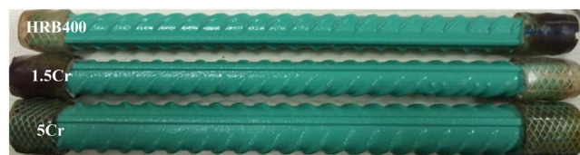
Fig. 15. Corrosion morphology of the three kinds of rebar covered with ordinary epoxy coatings after the removal of concrete layer.
