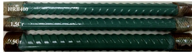
Fig. 16. Corrosion morphology of the three kinds of rebars covered with high-performance epoxy coatings after the removal of the concrete layer.
