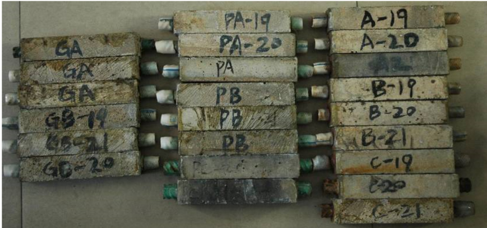
Fig. 12. Macromorphology of rebars after a 1-year field test in the splash zone in Zhanjiang.
