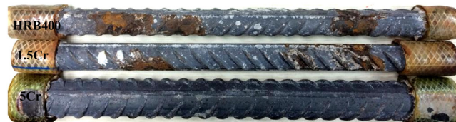
Fig. 13. Corrosion morphology of three kinds of bare rebar after a 1-year field test in the splash zone in Zhanjiang.
