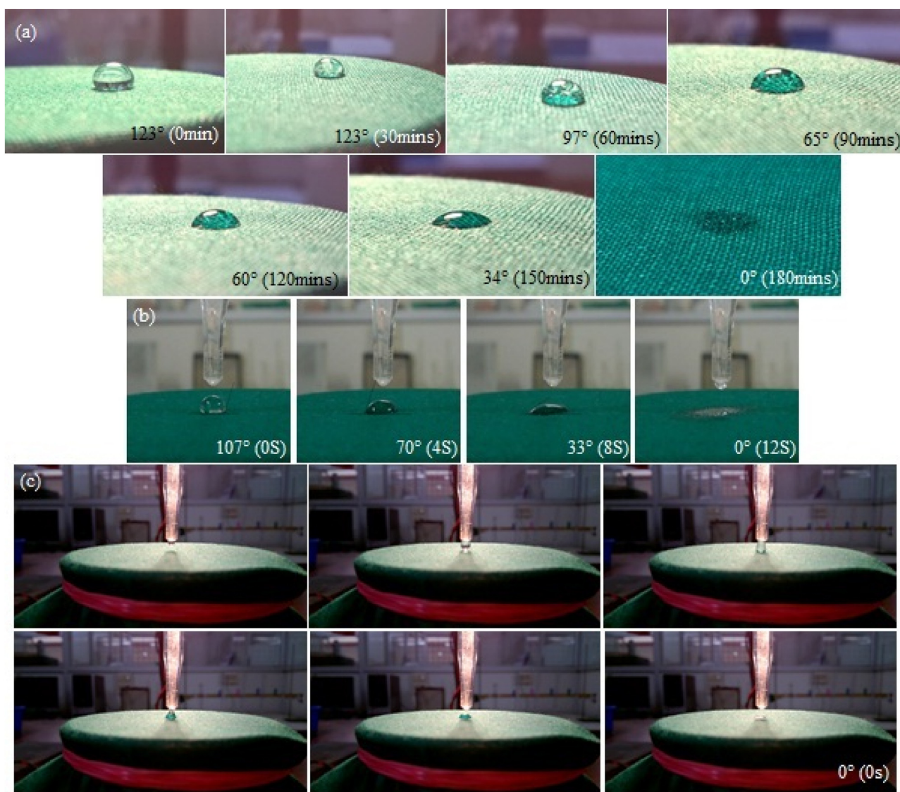
Fig. 4. Water Contact angle (a) sample with impaired hydrophilicity (b) control and (c) sample with improved hydrophilicity.
