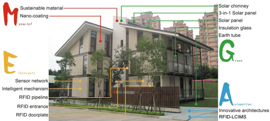
Fig. 2. Creative and intelligent open-building MEGA House.
