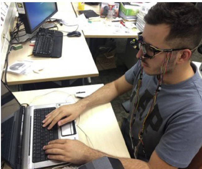
Fig. 3. A male participant wearing the glass frame with infrared sensing system.
